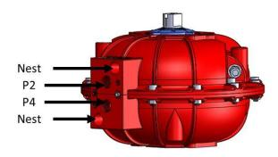
Port 2 and port 4 pass to the vane chamber, the nest holes are connected to the air reservoir chamber. Pressure entering port 4 rotates vane clock wise, pressure entering port 2 rotates vane counter-clockwise.
