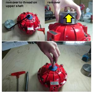
Caution: Ensure plenty of threading is engaged between upper shaft and shaft puller to prevent threads from being stripped.
