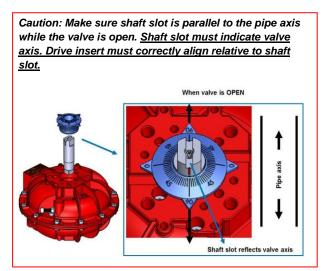
Install upper shaft and blue graduated ring back into actuator.
